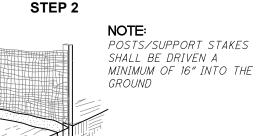
BACKFILL AND COMPACT THE EXCAVATED SOIL.
