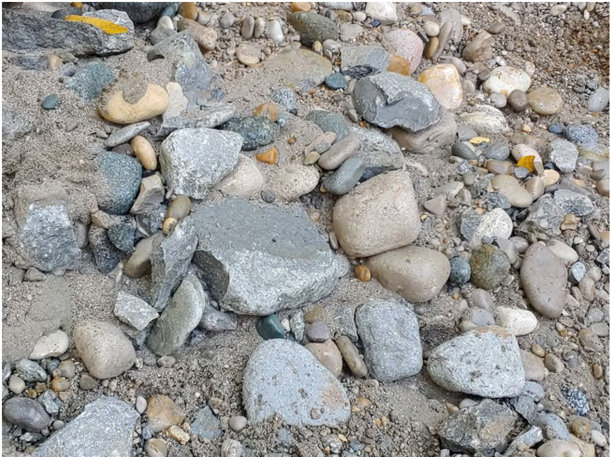
Cobbles and small boulders within the sand and gravel outwash at MJ-PW01.
