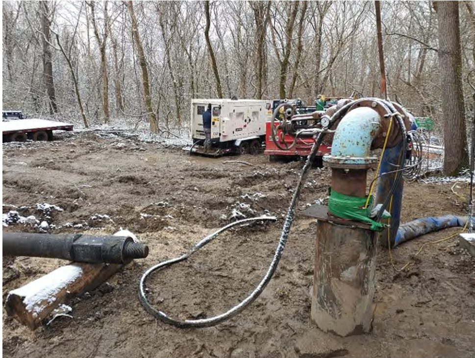
Figure 11. MJ-PW1 wellhead monitoring and flow control for SDT, CRT and RT.
