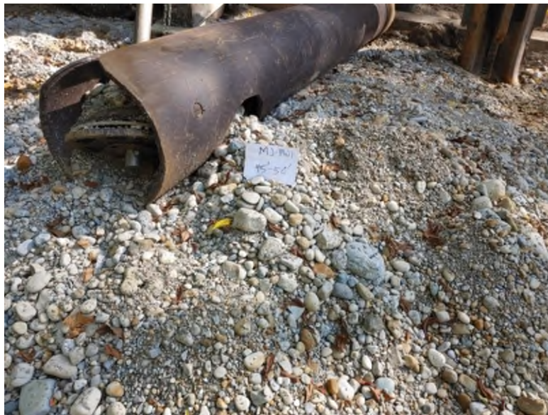
Figure 3. Course cobble outwash sand and gravel as found at MJ-PW1, September 2024.
