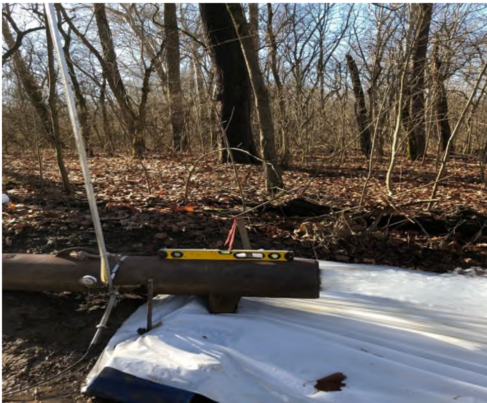
Figure 12. SDT & CRT discharge pipe, orifice and manometer to measure discharge.
