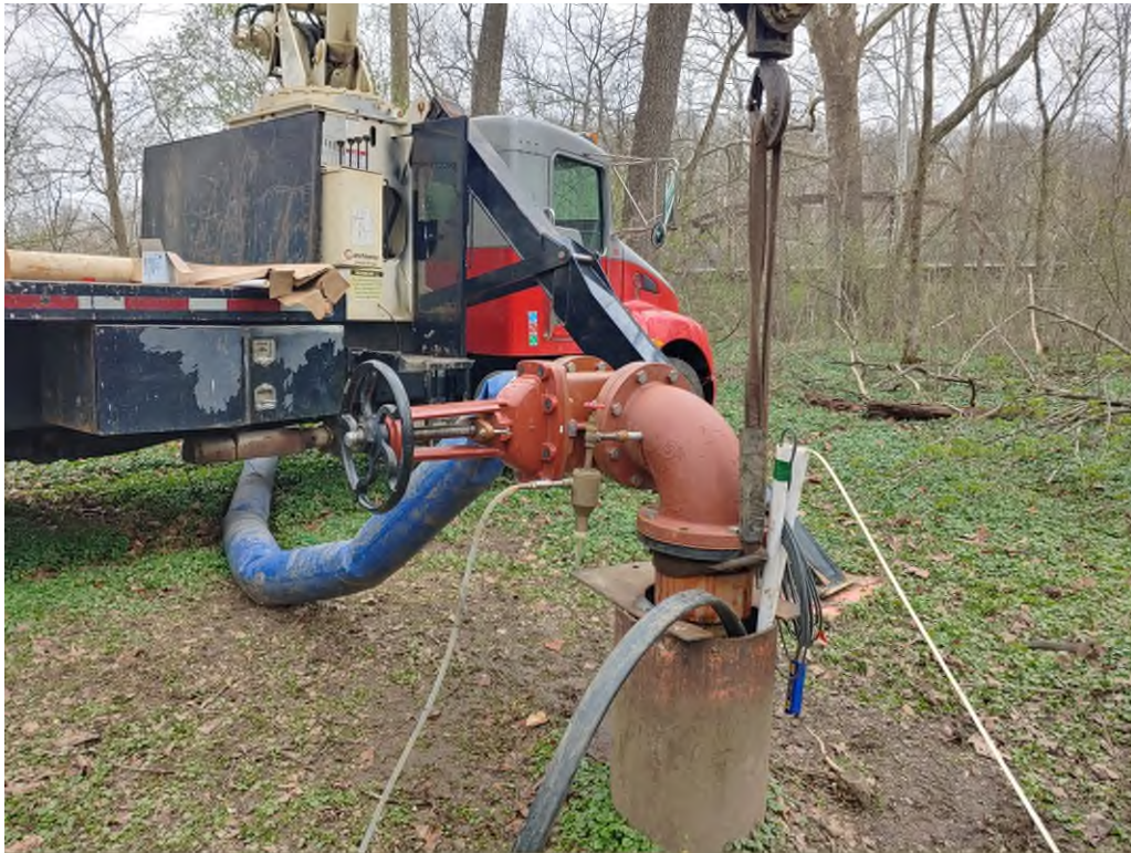
Figure 6. MJ-PW2 wellhead monitoring and flow control for SDT, CRT and RT.
