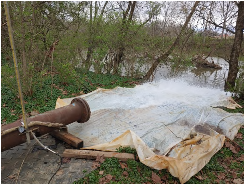
Figure 7. SDT & CRT discharge pipe, orifice and manometer to measure discharge.
