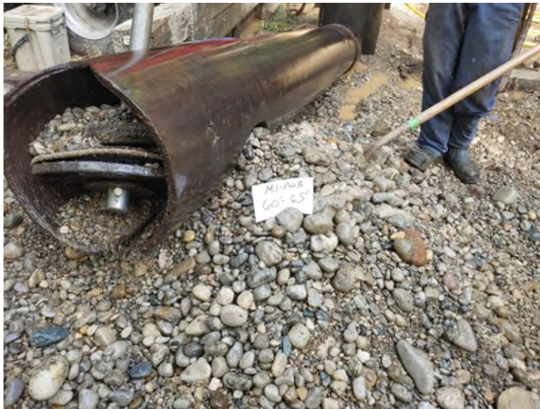
Figure 3. Coarse cobble outwash sand and gravel as found at MJ-PW3, August 2024.
