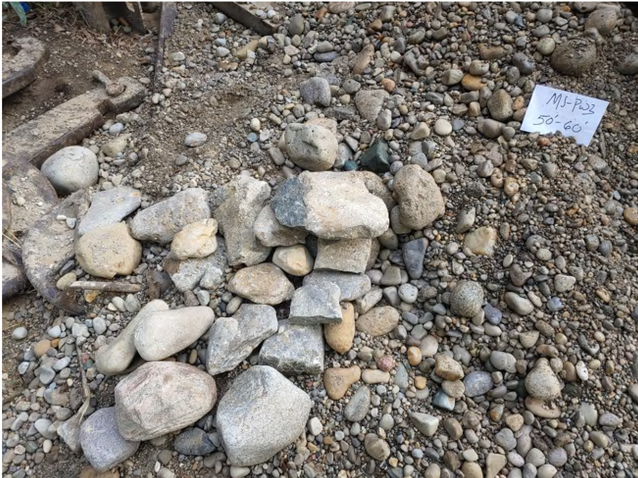
Coarse cobbled gravel outwash as encountered at production well MJ-PW3.
