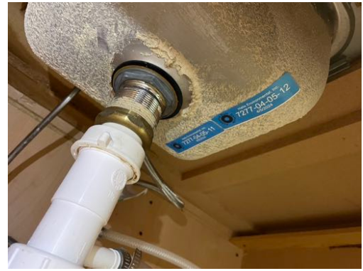
Photo 48- Sample# 7277-04-05-12, No Asbestos Detected in Sink Soundproofing
