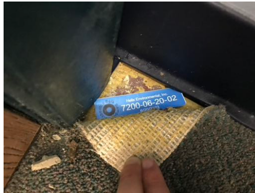
Photo 23- Sample# 7200-06-20-02, No Asbestos Detected in Tan Carpet Mastic, Asbestos Floor Tile Beneath
