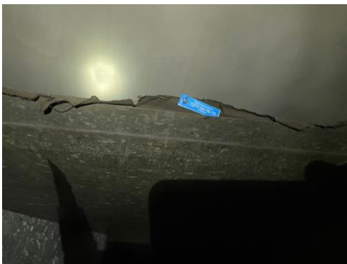
Photo 70- Sample #7277-04-16-10, No Asbestos Detected in Vibration Isolator Cloth
