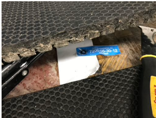
Photo 11- Sample# 7200-05-30-12, No Asbestos Detected in Faux Wood Stick on Floor Tile
