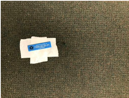
Photo 22- Sample# 7200-06-20-01, No Asbestos Detected in Tan Carpet Mastic, Asbestos Floor Tile Beneath
