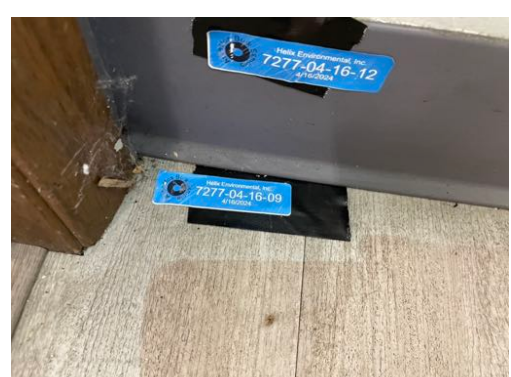
Photo 69- Sample #7277-04-16-09, No Asbestos Detected in Flooring
